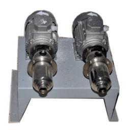
The oil transfer pump transports oil from the vibrating sieve to the centrifuge, and from the oil tank to the clarifiers or reservoir. The units are equipped with balustered spindles in a stainless-steel body and a food-grade elastomer stator with high abrasion resistance.
