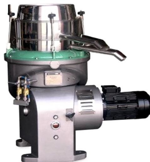
Self cleaning, Open type. Product feeding as well as the outlet oil and water phases are performed by gravity.
